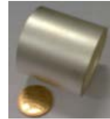
Tubular transducer typically operated at 69 kHz
